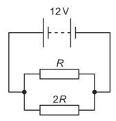
The total power dissipated by the two resistors is 36 W.
