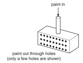
The paint is ejected at a speed of  $2.5\,\mathrm{m\,s^{-1}}$  through 400 holes, each of area  $0.4\,\mathrm{mm^2}$ . The density of the paint is  $900\,\mathrm{kg\,m^{-3}}$ .
